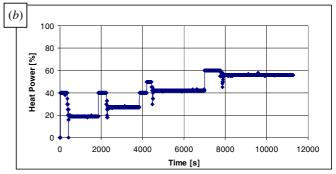
**Figure 7.** Engin-X inert-gas furnace output: (*a*) temperature and (*b*) heat output versus time on the P91 steel (9% Cr, 1% V) tensile specimen.
