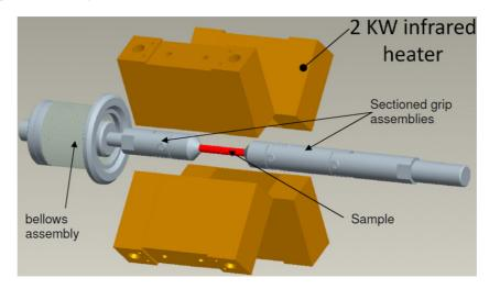
Figure 3. The experimental sample mounted between sectioned grip assemblies of stress rig and four 2 kW infrared heaters, positioned such that their focal zones coincide with the sample.
