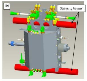
**Figure 4.** The aluminum frame that locates the heaters in position on the stress rig. (a) The assembly with all the fittings added for cooling water and power for the heaters, sensors and inert-gas feedthrough and (b) the complete assembly attached to the cross-beams of the stress rig (shown in red).
