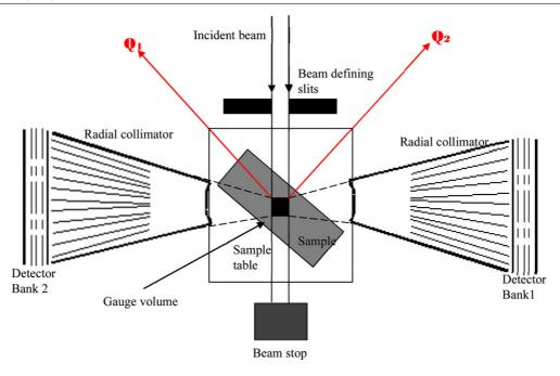
**Figure 1.** ENGIN-X experimental setup for *in situ* strain scanning. (Note that incident slits and collimators provide constrains to the maximum design size of the furnace.)
