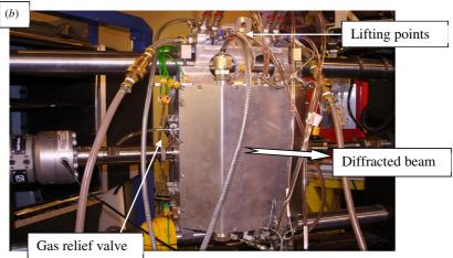
Figure 6. Engin-X inert-gas furnace overview of the experimental setup during the experiment: (a) incident beam side and (b) beam stop side.
