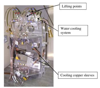
**Figure 5.** ENGIN-X inert-gas furnace off beamline, showing a compact easy-to-access assembly with lifting points cooling system providing cooling water to the lamps and cooling sleeves on the stress-rig grips.
