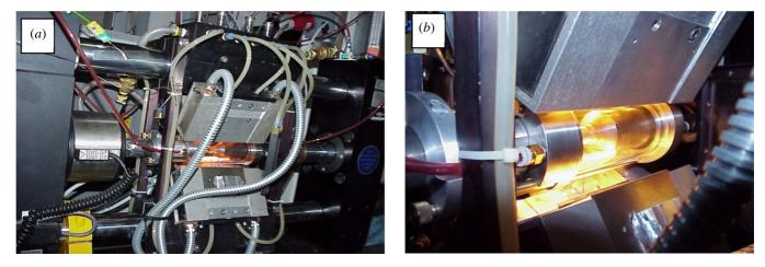
**Figure 2.** Photographs showing the previous method of providing inert atmospheres for the Engin X furnace: (*a*) overview of the setup and (*b*) close-up of the sample area and the glass canister.
